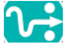
Figure 1. Feed Button. The button is helpful to advance label stock and activate other printer functions.
