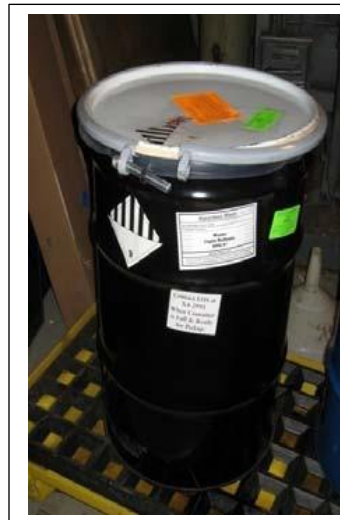
Figure 4. DOT-Approved Steel Drum With Lid. The drum is labeled with appropriate identification and shipment labels.
